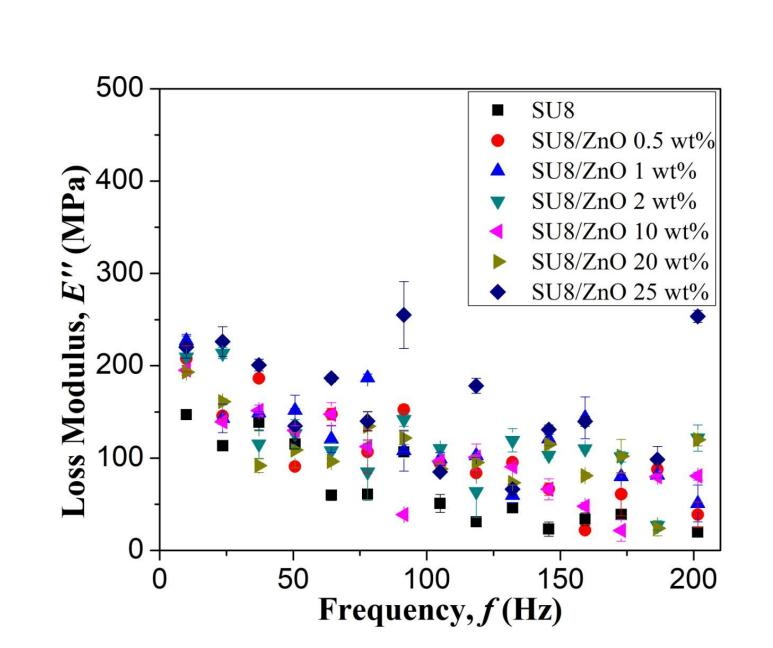
■ Dynamic nanoindentation (nano-DMA) results show that the SU8/ZnO nanocomposites exhibit viscoelasticity at room temperature in the frequency range of 10Hz to 201.5 Hz.
