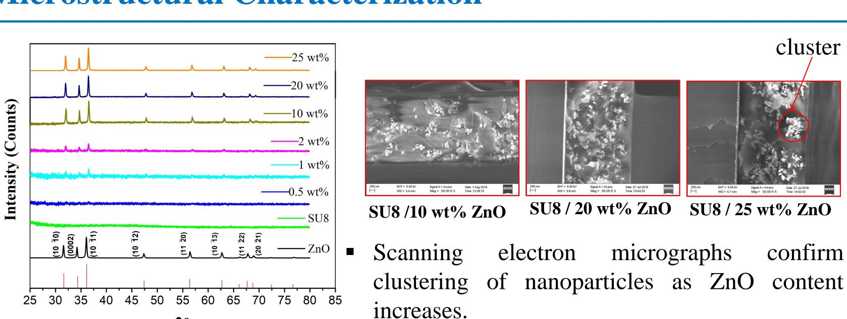
The integration of ZnO nanoparticles into SU8 produces neither new diffraction peak nor a peak shift, showing that ZnO nanoparticles filled SU8 composite consists of phase separated structures, i.e., polymer SU8 and ZnO nanoparticle.
